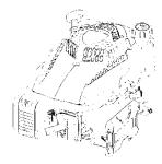
5) When mounting a new spark plug, you should screw 1/2 more thread with the wrench after the washer is compressed. If you are mounting an old one, you should only screw 1/8-1/4 more thread.
