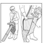
**IMPORTANT** When used as a vacuum collector not collect damp grass or leaves to avoid clog ging the rotor and coil.
