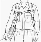
WARNING! The harness must always be worn when working with the machine. Failure to do so means you will be unable to manoeuvre safely and this can result in injury to yourself or others.
