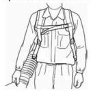
WARNING! The harness must always be worn when working with the machine. Failure to do so means you will be unable to manoeuvre safely and this can result in injury to yourself or others.
