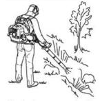
Engine speed should be adjusted to the type of material to be removed, it is seldom necessary to use full throttle, and many work procedures can be done at half throttle:
