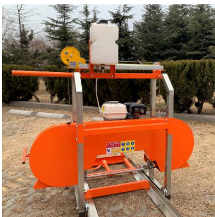
Operators side is on side with the scale stick and hand winch.
