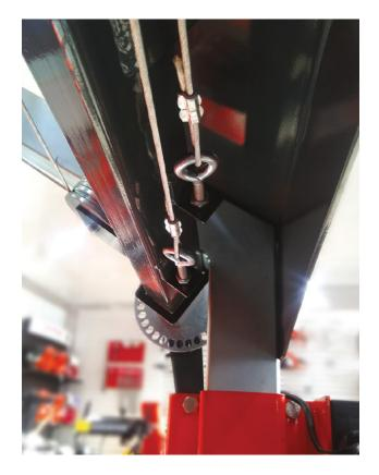
Add waterproof grease to the threads of the blade tension "T" handle and to the face of the washer before use. Proper blade tension is achieved when a 24mm socket is used on a torque wrench to tighten the handle to 17nM (12.5 ft lbs, 150 inch lbs). See pictures below.
