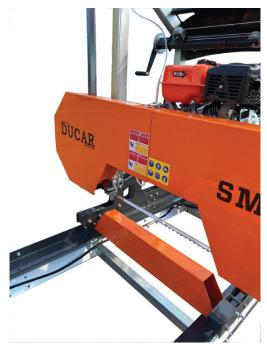
Push the saw head forward and back of the rail system to ensure that the width of the rail allows the saw head to move freely. If it binds or feels tight, the cart wheel spacing can be re-adjusted by adding or removing washers.
