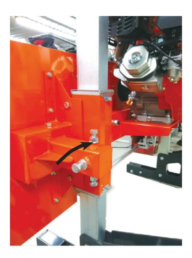
Wearing gloves, spin the wheel with your hand and see the changing path of the blade. Measure the distance again and repeat the steps above to compensate further if needed. The best measurement possible is 10mm (3/8") or check that the back of the blade is aligned with the back of the tape wheel.
