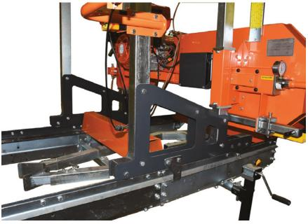
With the saw head nowin place on the track, all of the head screws can be tightened.
